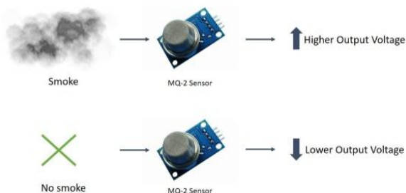
Figure 6 MQ-2 Gas Sensor
