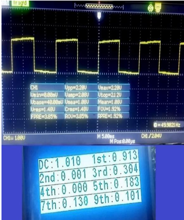
Figure 14 Harmonics calculations of square waveform on the microcontroller
