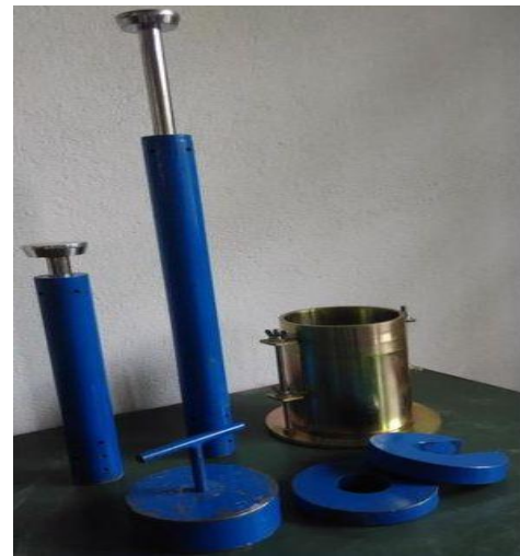
Figure 2: CBR mold with compaction hammers
