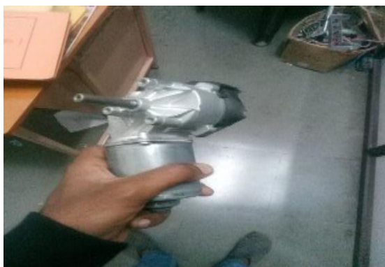
Figure 4 Conveyor motor with shaft and gear box
