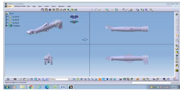
FIGURE 11 SHOCK STRUT DESIGNED IN CATIA
