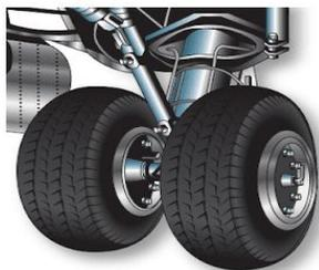
FIGURE 2 MAIN GEAR OF A TRICYCLE-TYPE LANDING GEAR
