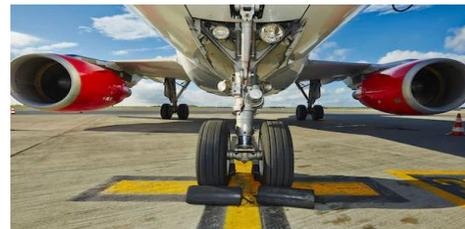
FIGURE 3 NOSE LANDING GEAR
