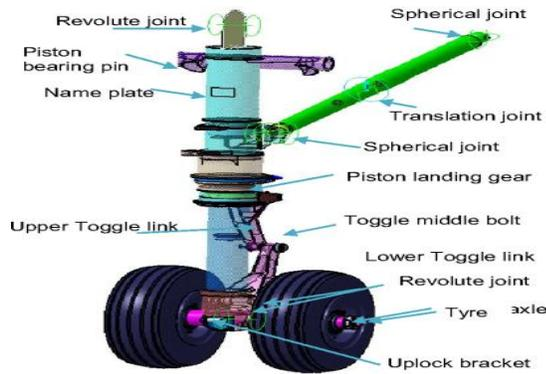
FIGURE 1 PARTS OF LANDING GEAR
