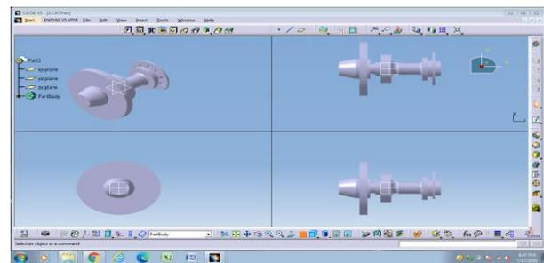
FIGURE 13 AXLE SHAFT DESIGNED IN CATIA
