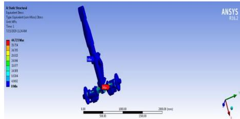
FIGURE 19 VON-MISSES STRESS OF TI 10AL-2FE-3V MATERIAL
