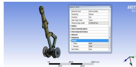
FIGURE 17 MESH : NODES:49344, ELEMENTS 25340
