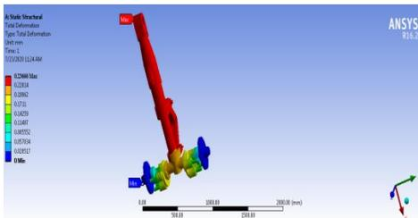
FIGURE 20 TOTAL DEFORMATION OF TI 10AL-2FE-3V MATERIAL
