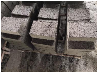
fig.4 Bricks placed for Curing
