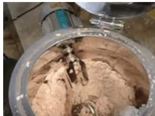
Figure 1.1: PVC powder mixing
