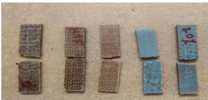
Figure 9 Impact test Specimens before testing
