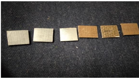
Figure 6 Hardness test Specimens before testing
