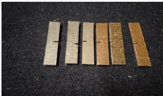
Figure 7 Impact test Specimens before testing
