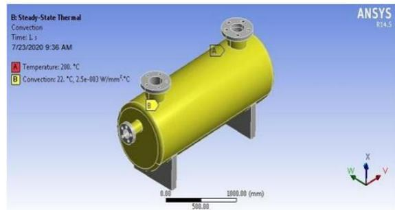
Figure 9 Boundary condition of flat head pressure vessel in Thermal analysis
