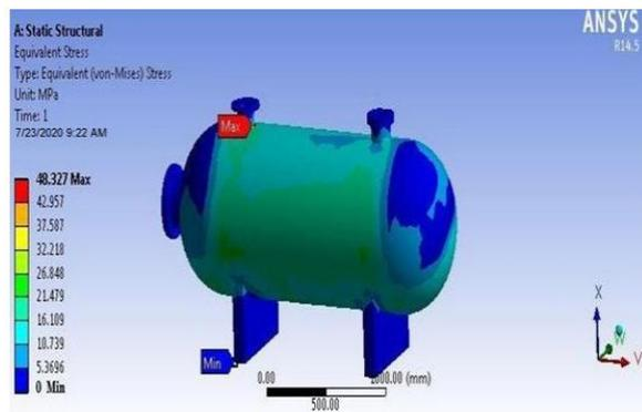
Figure 11 Von-mises Stress on Elliptical head
