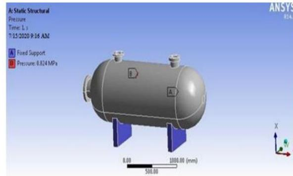
Figure 10 Boundary condition of Elliptical head pressure vessel in static analysis
