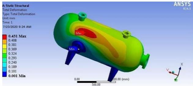
Figure 12 Total deformation on Elliptical head
