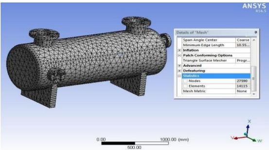
Figure 7 Mesh of flat head
