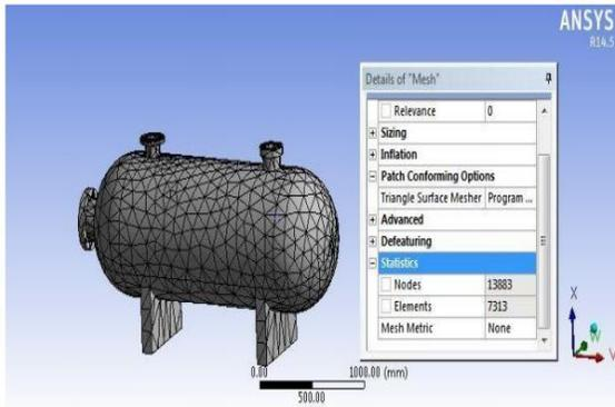
Figure 6 Mesh of Elliptical head
