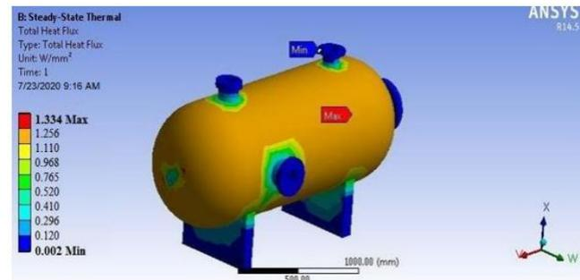
Figure 13 Heatflux on Elliptical head
