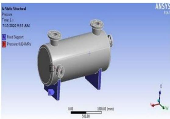
Figure 8 Boundary condition of flat head pressure vessel in static analysis
