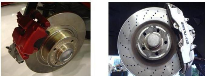
**Fig1:Disk brake without holes & disk brake with holes**
