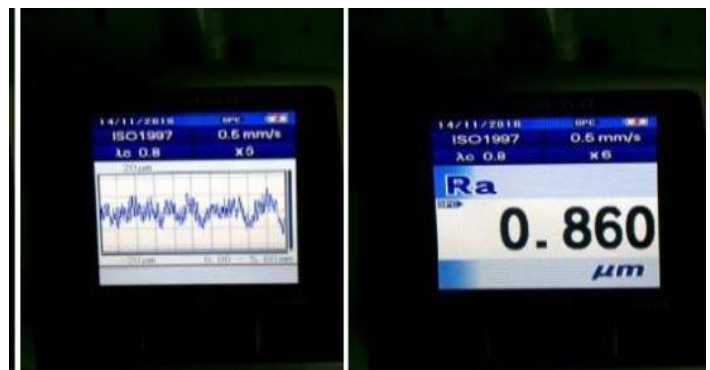
Fig 4.5: Testing of surface roughness
