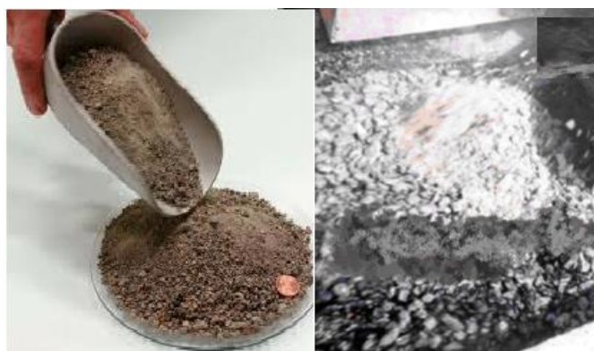
Figure 5 : Adding BA into bitumen
