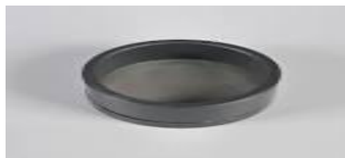
Figure 3. 1 90 micron sieve for fineness test.
