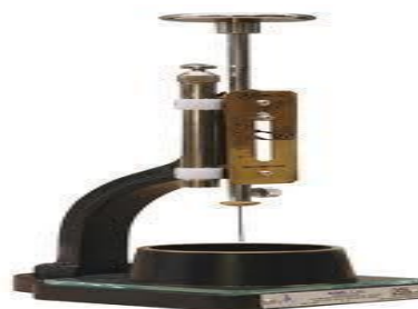
Figure 3. 2 Vicat Apparatus for Consistency, IST, FST.
