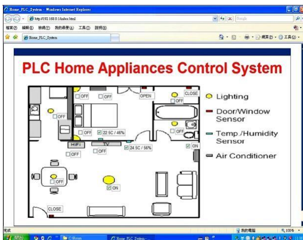
Fig. 14 PLC home appliances control via Internet browser
